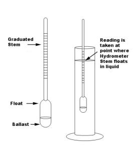
To monitor the level of borates in the treatment solution, the EBF manual recommends using a **salt measuring hydrometer** "under normal temperatures of your region" as opposed to measuring during either extreme hot or cold weather conditions. We have found that the optimum air temperature range to measure the solution is 20-25 degrees C (68-77 degrees Fahrenheit).
