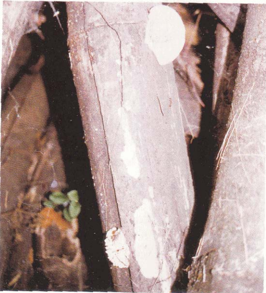
Figure 4: Soft rot of bamboo culms caused by Daedalia sp.
