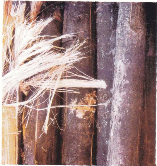
Figure 5: Soft rot of bamboo culms - advanced stage.
