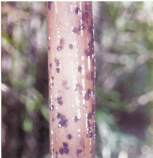
Figure 1: Surface moulds on bamboo culm.
