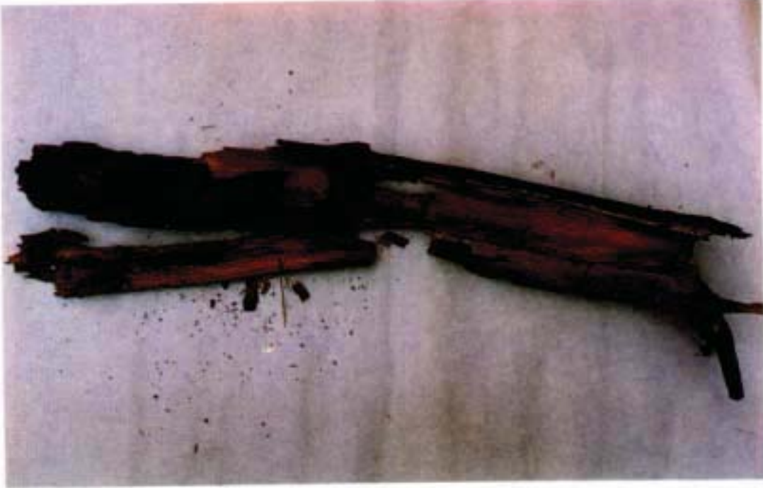
FIGURE 3(a). Advance decay and insect attack in Bamboo.
