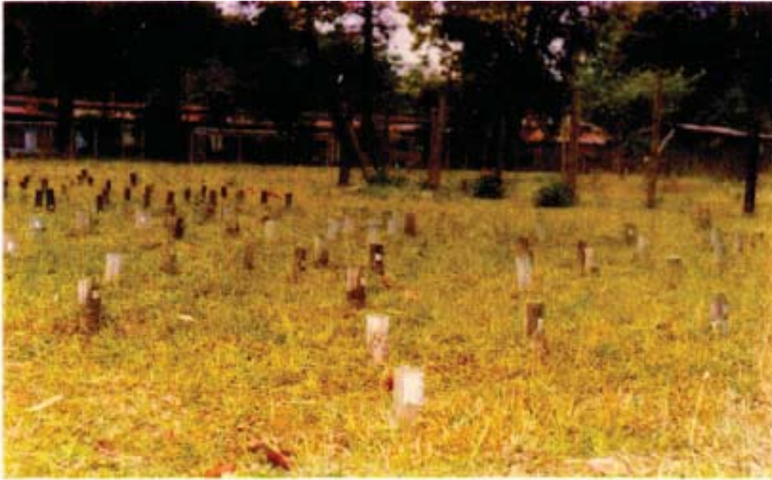
FIGURE 1. Graveyard tests on treated and untreated bamboos
