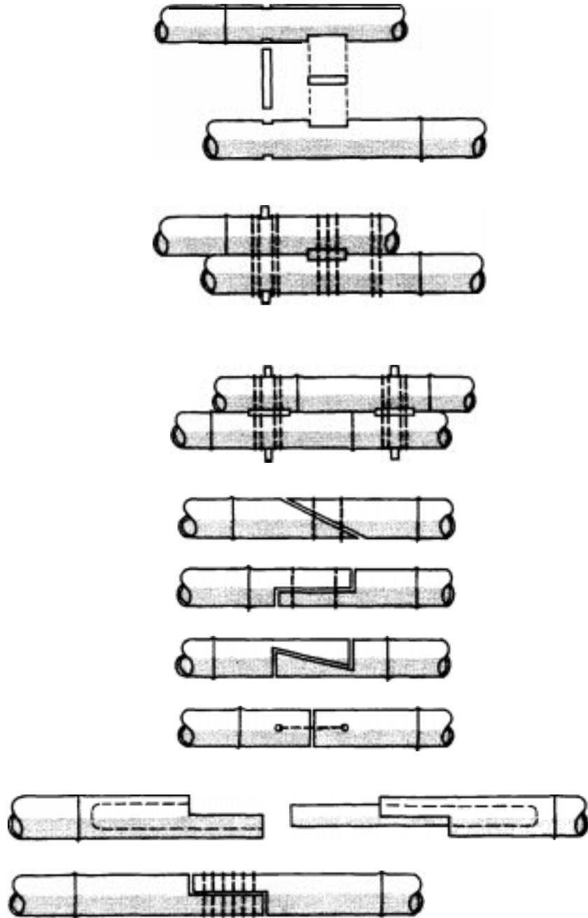
Figure 52: Variations on splice joints
