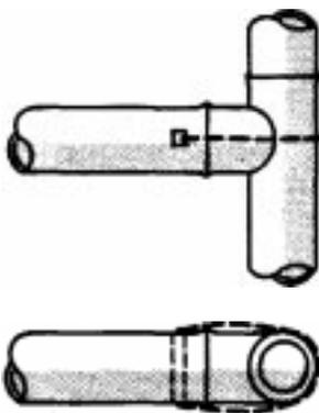
Figure 56: Saddle detail applied to horizontal framing
