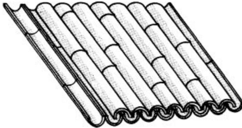
Figure 22: Roof of halved bamboo culms
