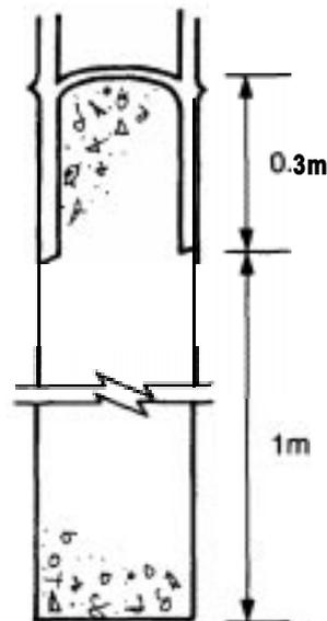
Figure 8: Composite bamboo/concrete column
