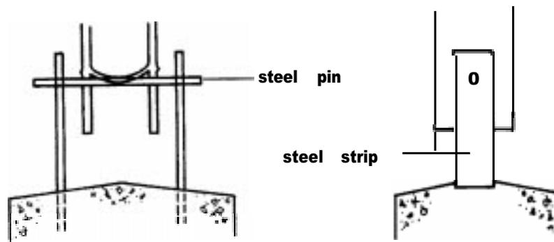
Figure 36: Arrangement for interchangeable post ends
