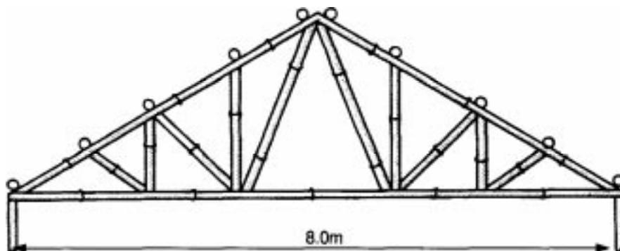
*Figure 26: Janssen (1995) truss configuration
