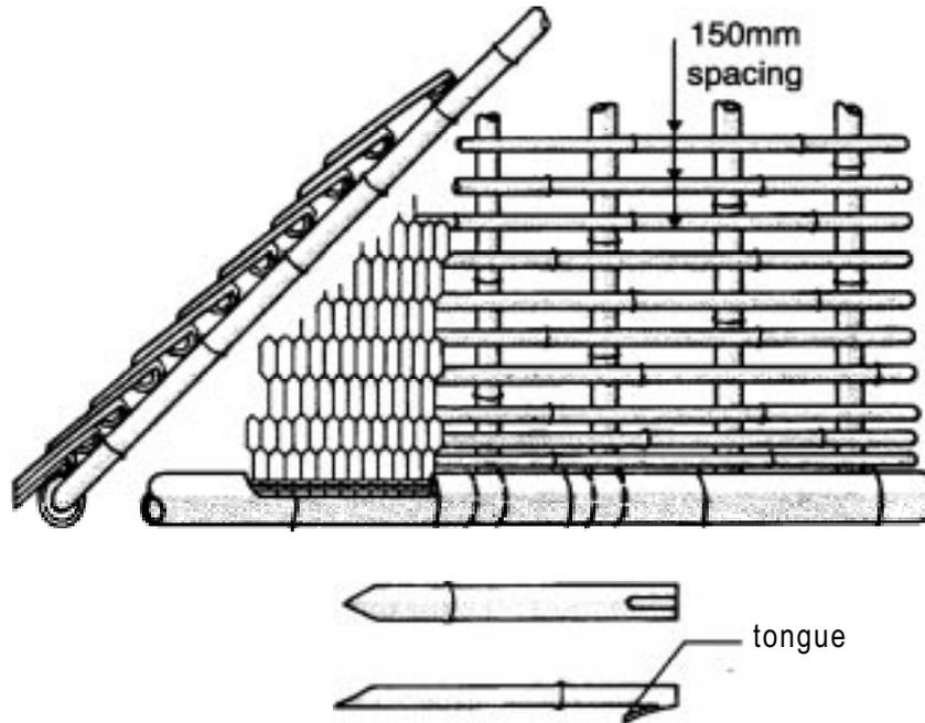
Figure 28: Bamboo shingles
