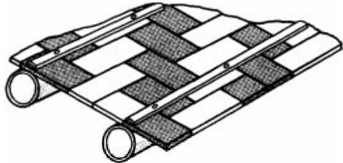
Figure 16: Woven bamboo mat floor decking
