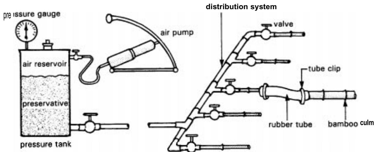
Figure 4: The modified Boucherie apparatus (after Nienhuys, 1976)
