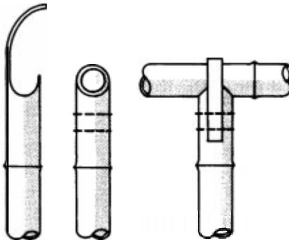
Figure 54: Saddle joint with tongue
