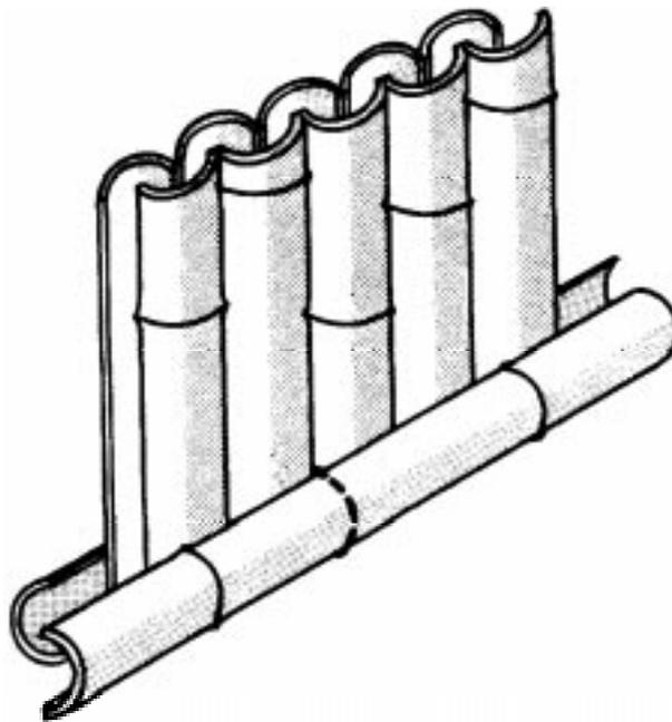
Figure 18: Wall of vertical halved culms
