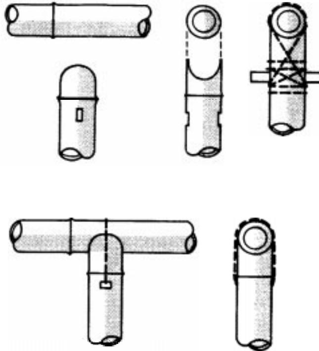
Figure 53: Saddle (butt) joint
