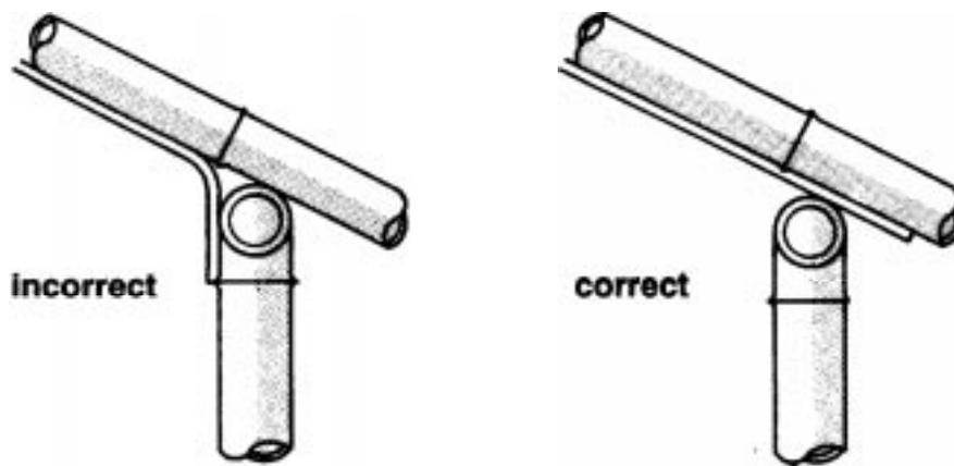
*Figure 38: Preferred ceiling (sarking) detail*
