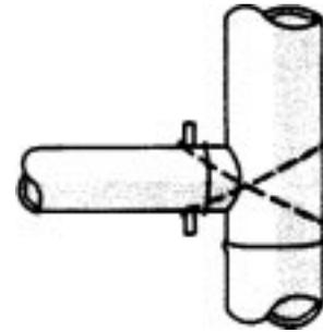
Figure 66: Example of doweled and tied joint
