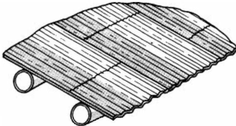
Figure 14: Flattened bamboo floor decking
