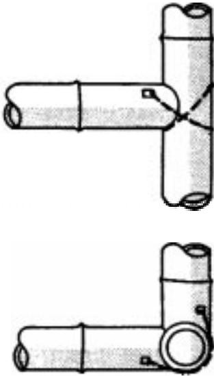
Figure 57: Double butt joint
