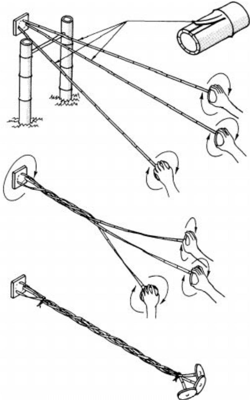
Figure 47: Bamboo cable reinforcement
