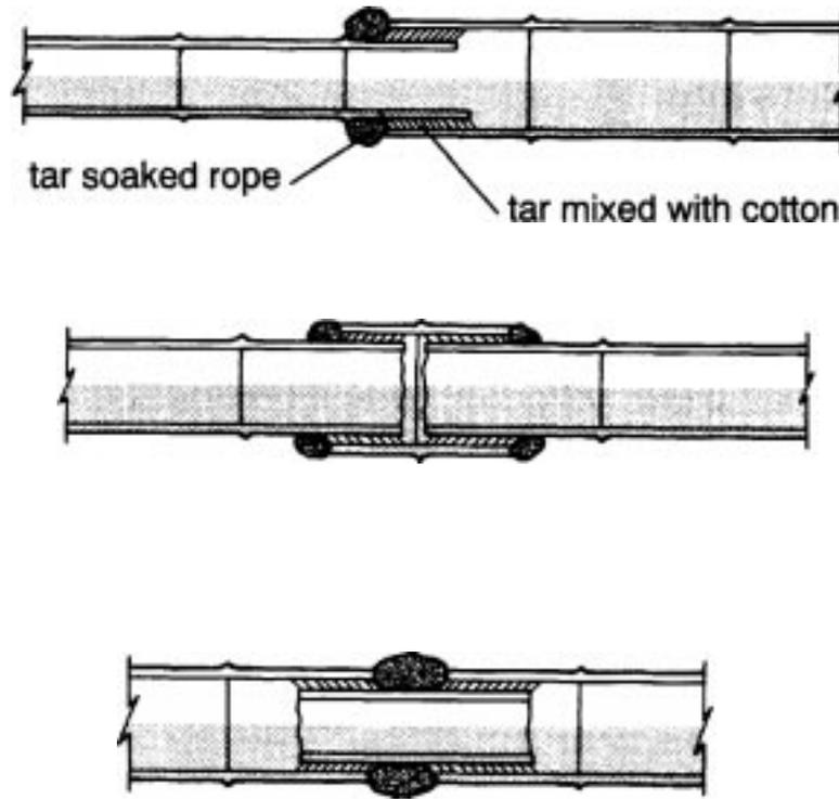
Figure 34: Jointing of bamboo pipes below ground
