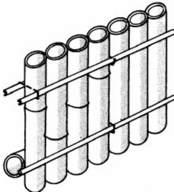
*Figure 17: Wall of whole bamboo culms
