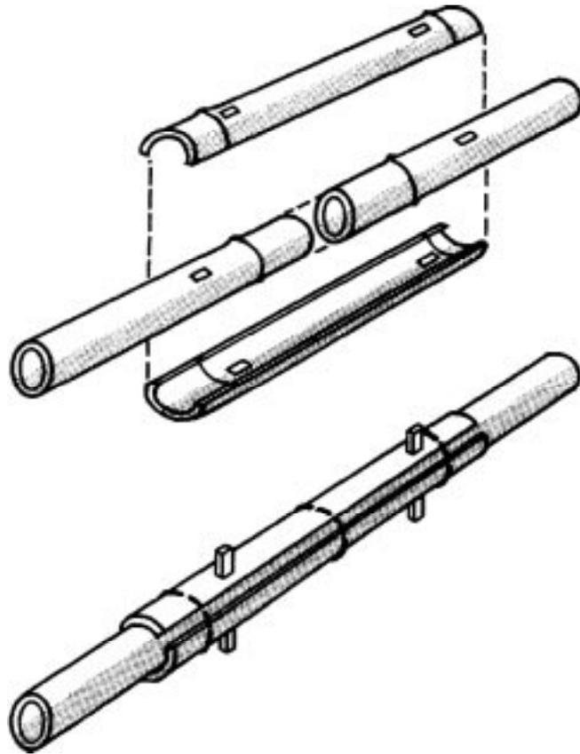
Figure 50: Butt joint with side plates
