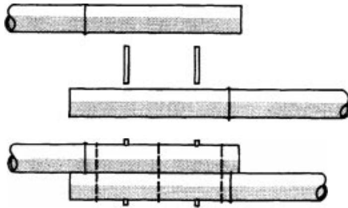
Figure 48: Full lapped splice joint
