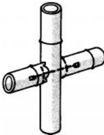
Figure 61: Insert joint
