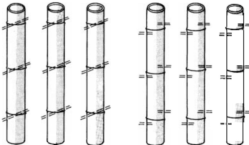
*Figure A2a: Boring pattern to puncture node*
