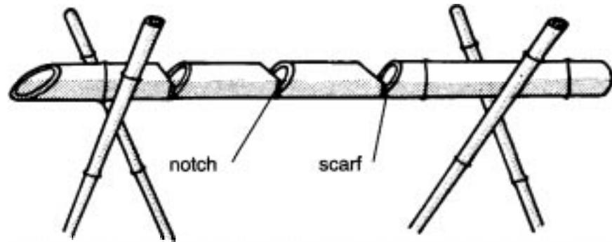
Figure 35: Bamboo piping above ground
