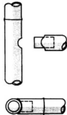
Figure 62: Beam supported on stump of branch
