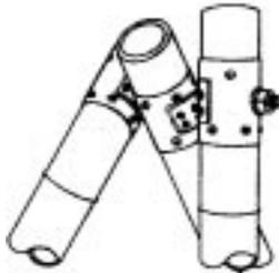
Figure 74: Herbert shear pin connector joint
