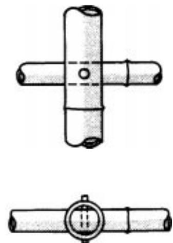
Figure 68: Through joint (after Stulz/Hidalgo, 1981)
