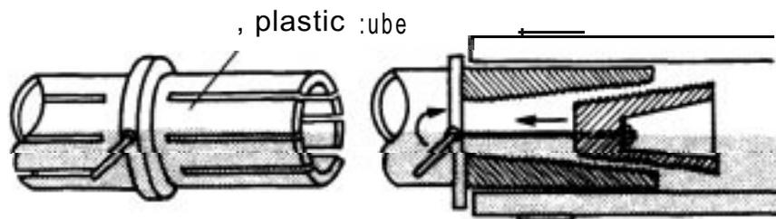
Figure 77: Expanding insert joint
