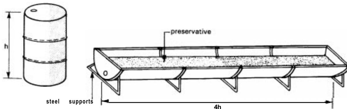
Figure 1: Open tank method for coid soaking
