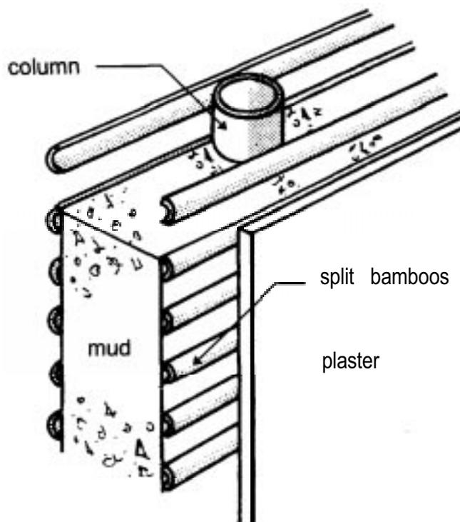
Figure 19: Bajareque wall construction
