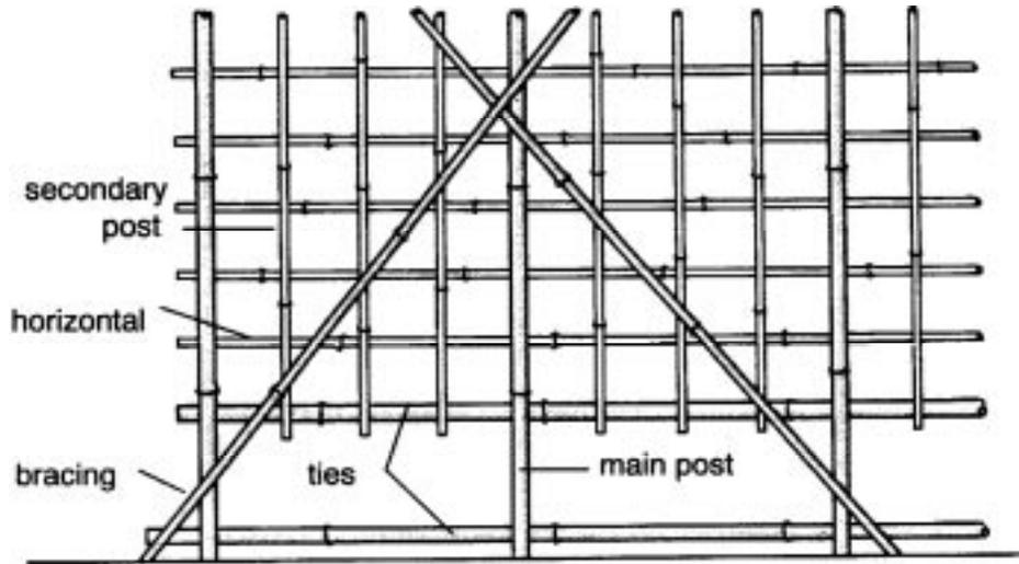
*Figure 45: Typical scaffolding arrangement
