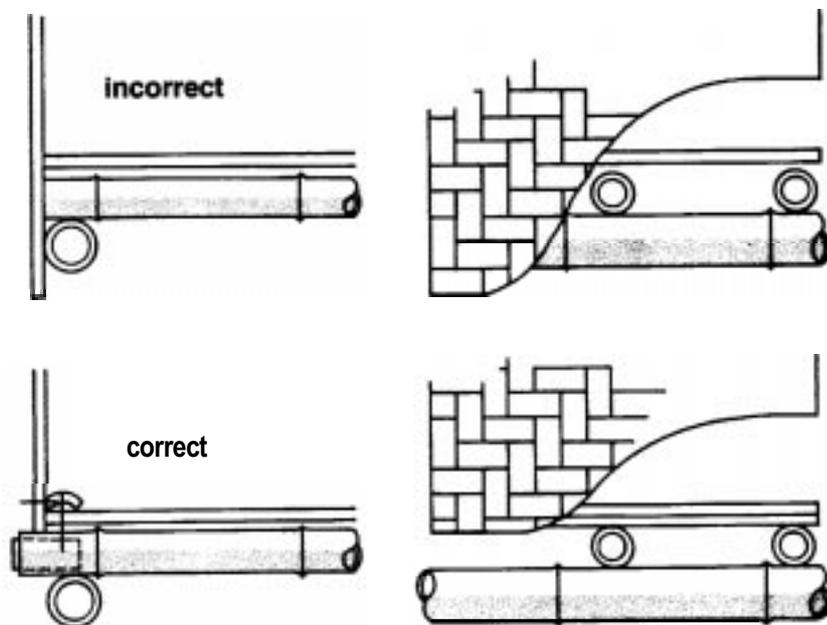
Figure 37: Preferred beam/joist end detail
