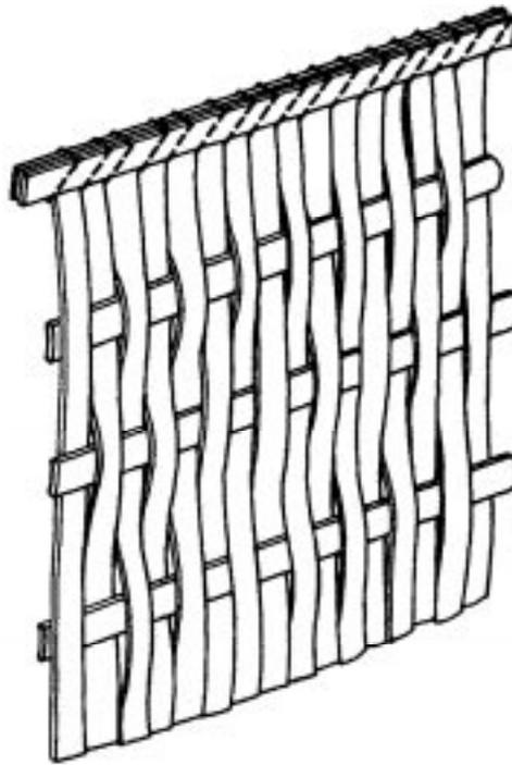
Figure 21: Woven bamboo wall construction
