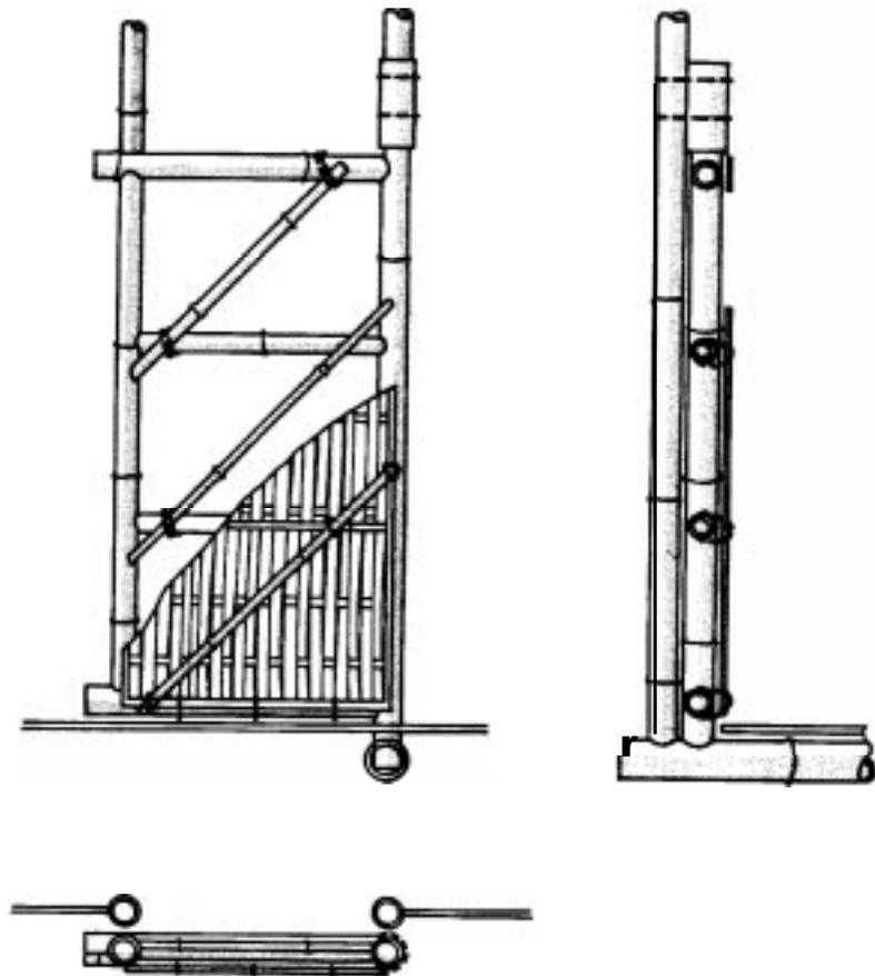
*Figure 30: Arrangement of hinged door
