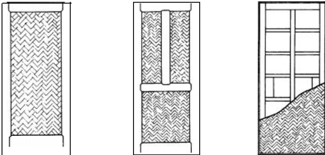
Figure 32: Bamboo mat board panelled and hollow core doors
