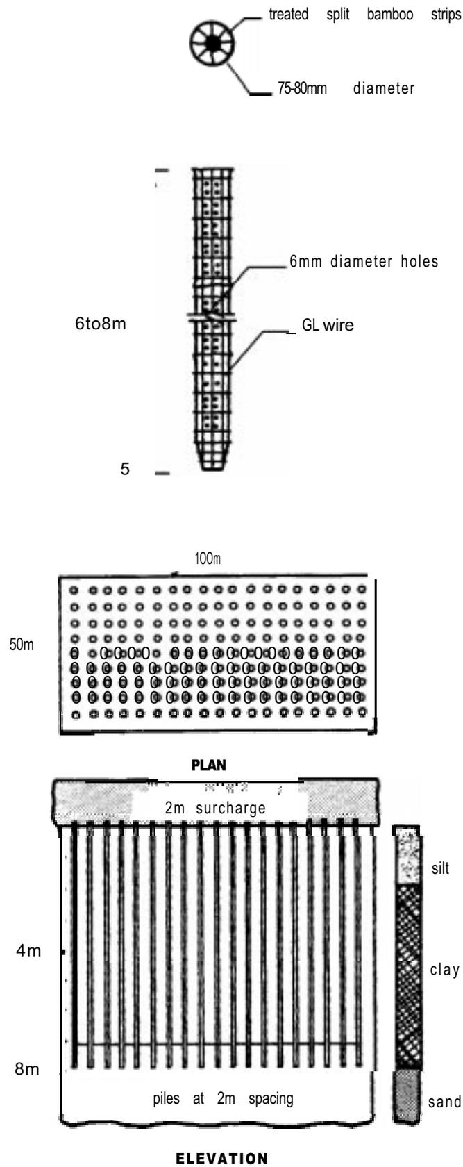
Figure 9: Bamboo piles (after Stulz/IGE, 1983)
