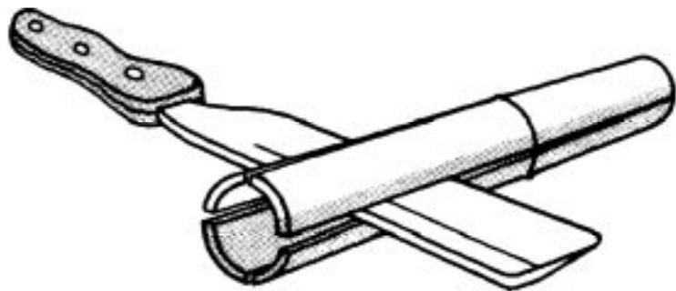
**Figure 79: Splitting knife for small culms (after McClure, 1953)**
