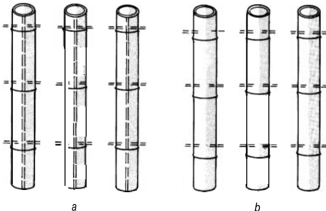
*Figure A 1: Boring pattern with nodes bored or knocked out*
