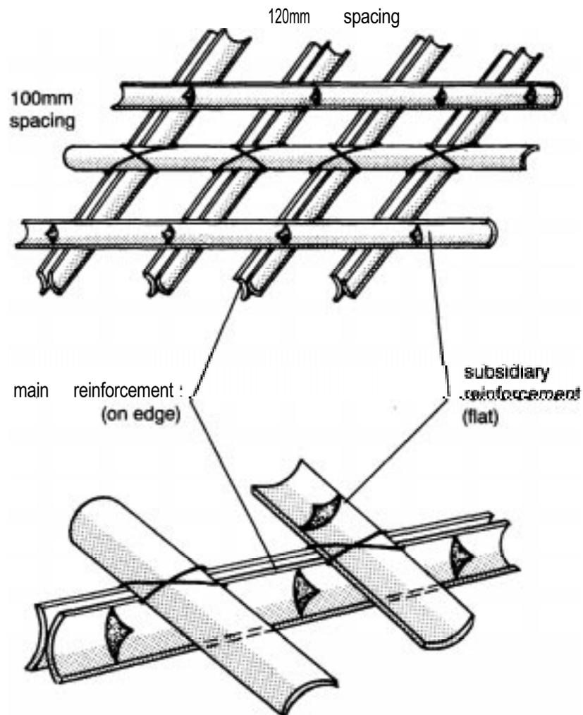
Figure 46: Bamboo strip reinforcement (FRI, India)
