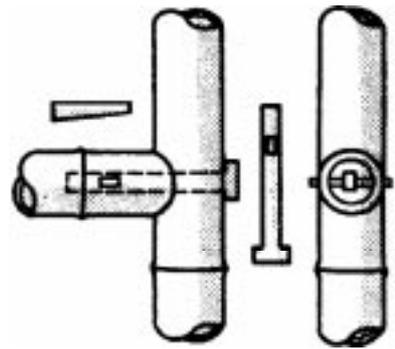
Figure 59: Tenon and key joint (after Stulz/Hidalgo, 798 1)
