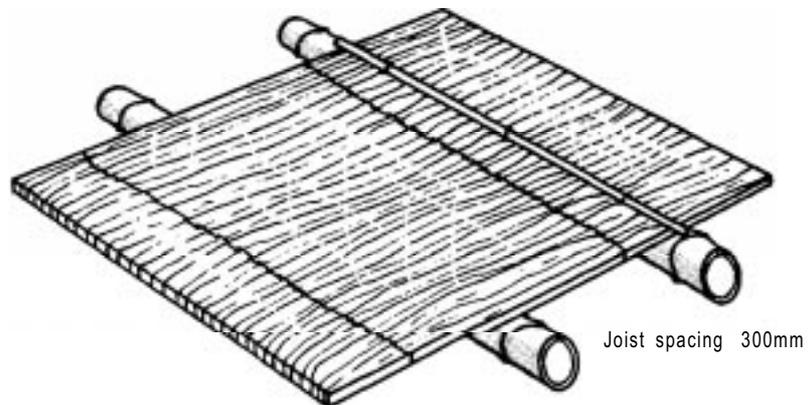
*Figure 10: Joist arrangement - primaries on/y
