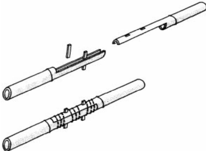
Figure 49: Half-lapped splice joint
