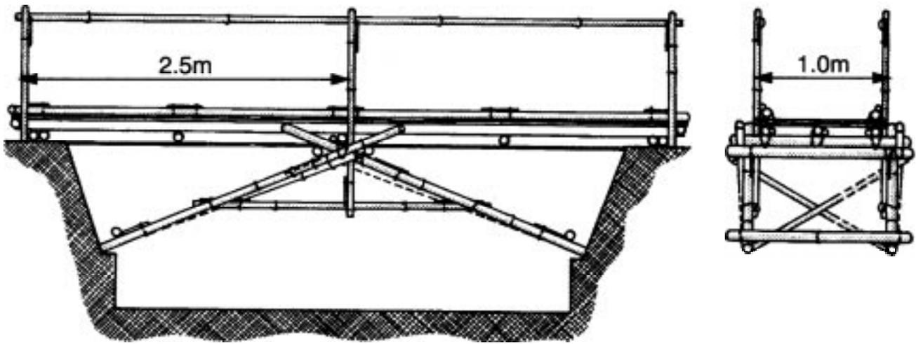
Figure 42: Simple truss (flying buttressed) bridge (after Janssen/Trojani, 1982)
