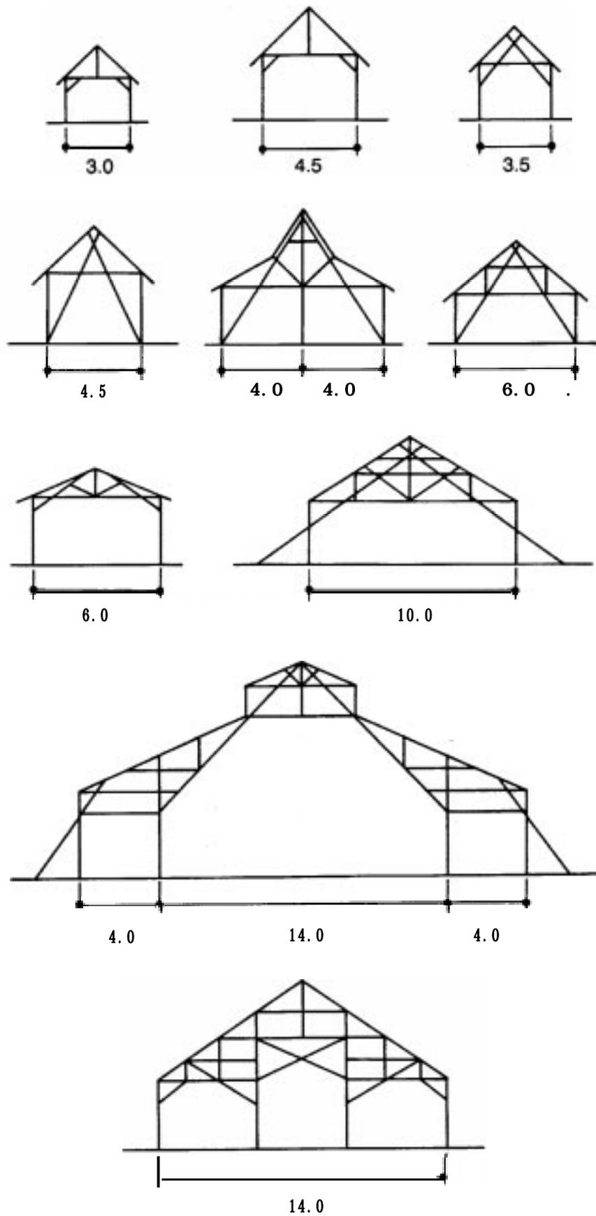
Figure 23: Possible roof framing configurations using traditional forms of construction - dimensions in metres (after *tular* et al. 1984 and Janssen, 1995)
