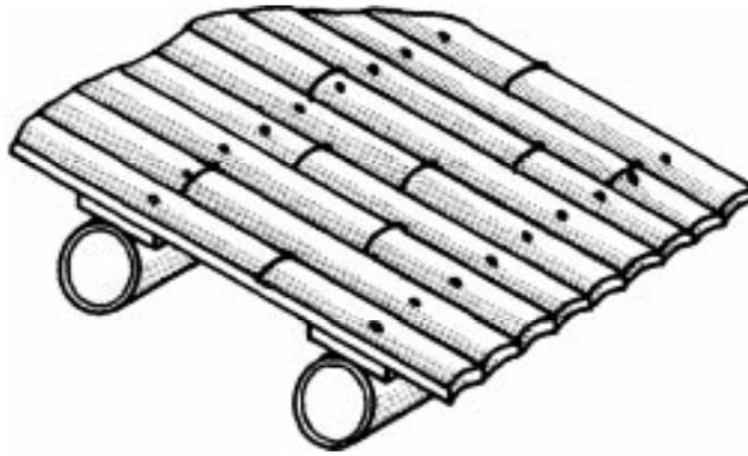
Figure 73: Split bamboo floor decking
