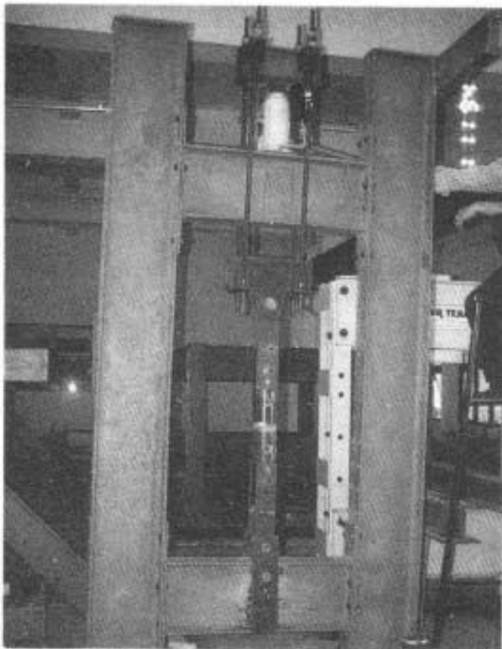
Fig. 2: Individual joint test
